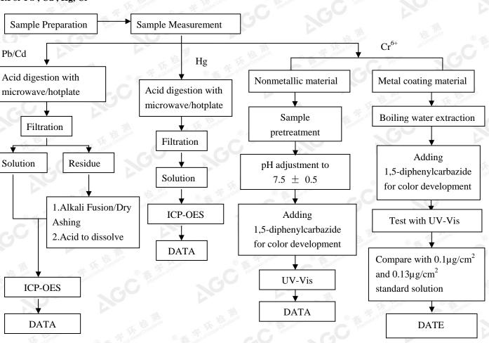
These sample were dissolved totally by pre-conditioning method according to above flow chart ( $Cr^{6+}$  test method excluded)
